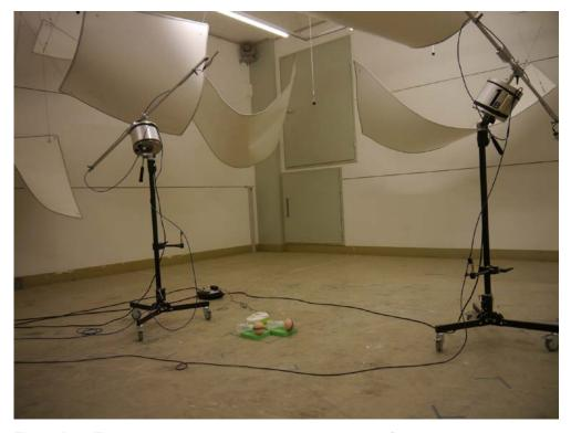
Figure B.3. Test arrangement on the reverberation room floor.
