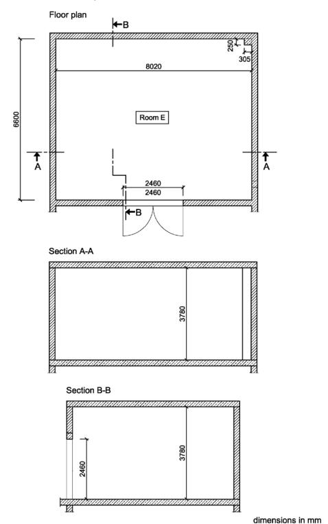
Figure D.1. Plan view and sections of the reverberation room.
